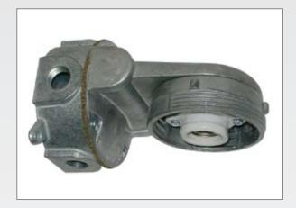
**SOCKET** Porcelain, medium base, 4KV pulse rated socket with a nickle-plated screw shell and a spring-loaded centre contact.
