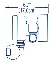
The MS-LED-1H-180 is equivalent to a 300 watt quartz unit with a total of 1800 lumens out of the fixture. Whenever the motion sensor detects motion the floodlight automatically turn on. The sensor is adjustable and can turn the light on from 5 seconds to 12 minutes.
