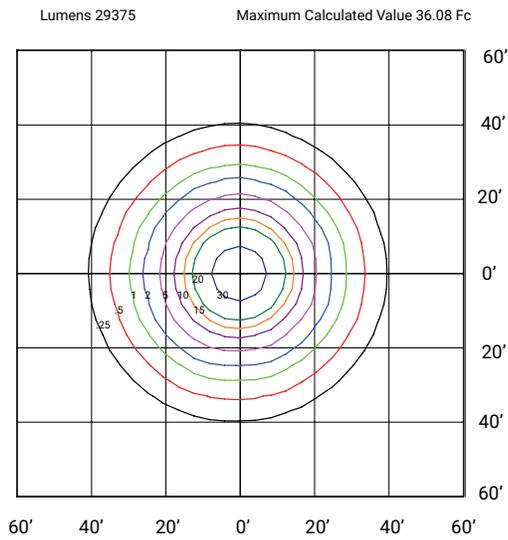
RH2S-LED240A200-H-VK-DIM-PCL-FS-N4X- POLYCARBONATE REFLECTOR (240W 4K)
